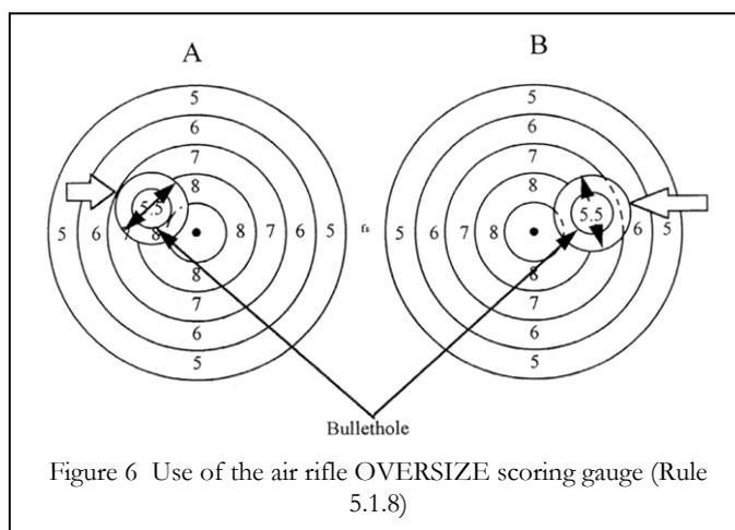
Figure 6 Use of the air rifle OVERSIZE scoring gauge (Rule 5.1.8)
