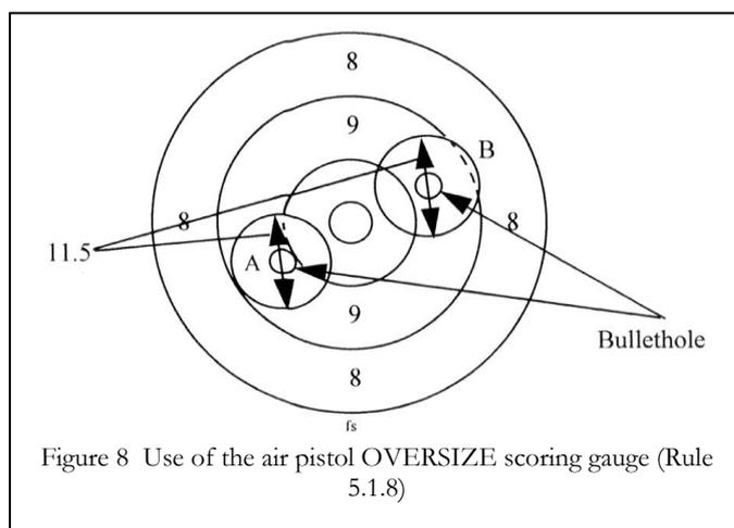
Figure 8 Use of the air pistol OVERSIZE scoring gauge (Rule 5.1.8)
