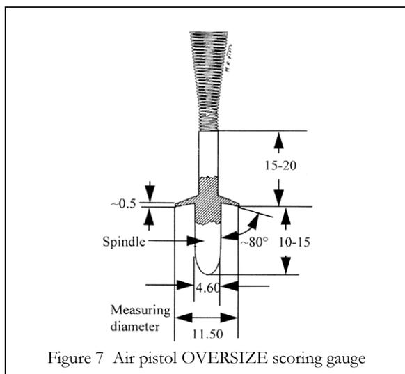
Figure 7 Air pistol OVERSIZE scoring gauge
