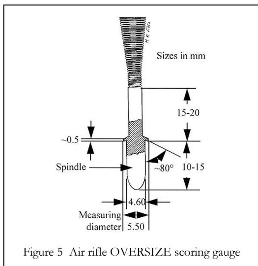
Figure 5 Air rifle OVERSIZE scoring gauge
